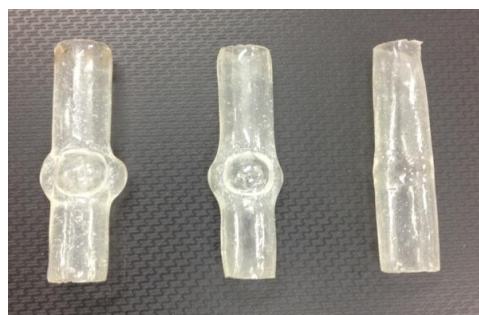
Fig. 12 Silicone ePTFE valve conduit model used for this experimental study: 1.0x Bulging sinus (left), 0.75x Bulging sinus (middle), 0.2x Bulging sinus(right) 6)
