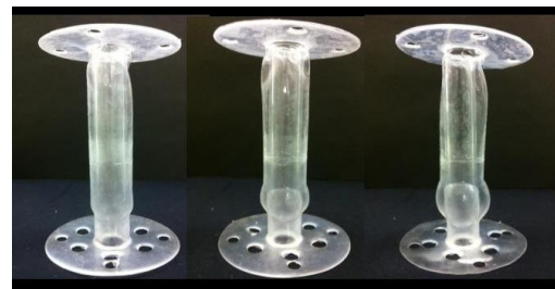
Fig.2 Photographs showing test aorta models used for this study: 50% Sinus of Valsalva (left), Normal Sinus of Valsalva (center), and 150% Sinus of Valsalva (right) 2)
