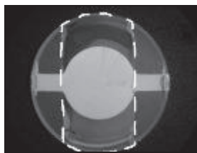
Fig.3 Crystal plate coated with acrylonitrile-styrene copolymer in the area enclosed with dotted line
