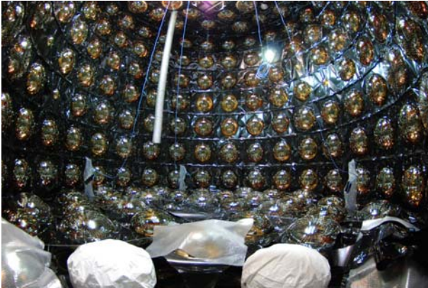
Inside of EGADS tank during PMT installation; August 2013.
