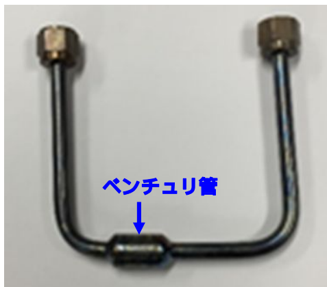
Fig.3 Structure of Venturi tube and photograph of a reactor for Cavitation + hydrothermal oxidation.
