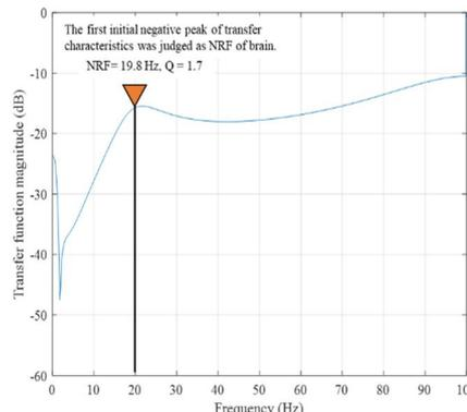
Fig.8 The graph for the relationship between transfer function magnitude and frequency. The first peak of transfer characteristics was judged as the NRF of the brain.
