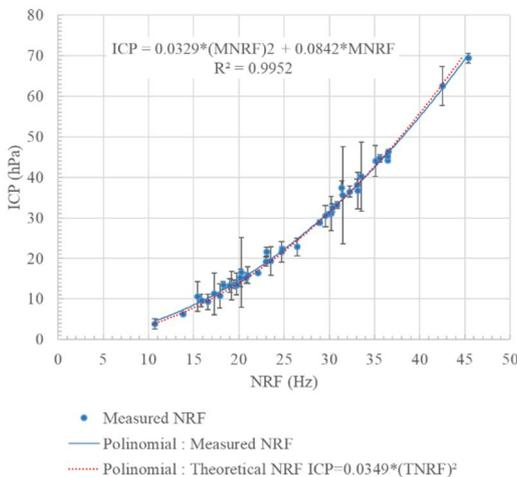
Fig.9 Blue points is plotted the relationship between the measured ICP value and the NRF of the brain. Error bars indicate SD. These parameters are strongly correlated with each other (R<sup>2</sup>= 0.999947). The blue polynomial: approximation graph from blue points. The red polynomial: theoretical calculation graph.
