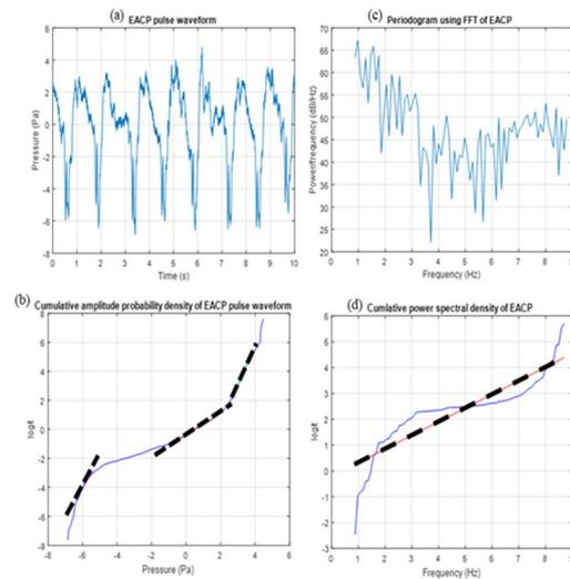
Fig.3 An example of the signal processing results. (a) : the EACP pulse waveform, (b) : the cumulative amplitude probability density, (c) : the periodogram using FFT, (d) : the cumulative power spectral density.
