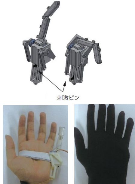
Fig. 2: top panel: the design of our sixth finger system. Bottom panels: the sixth finger device fixed on a users hand, with and with gloves.
