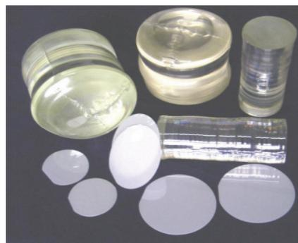
Fig.1  $\text{LiTaO}_3$  crystal and wafer
