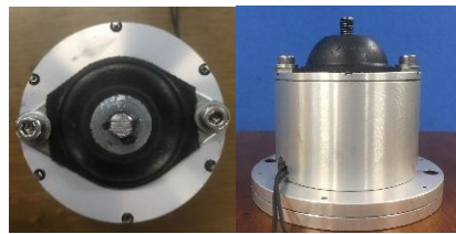
Fig.4 Vibration isolator incorporating MRC
