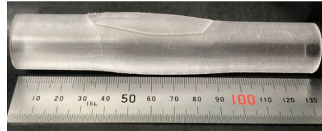
Fig. 2 3D-reconstructed vascular structure by photopolymerisation with an elastic membrane.
