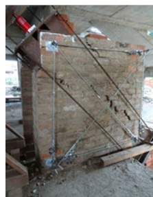
Photo.4 Diagonal Compression Test
