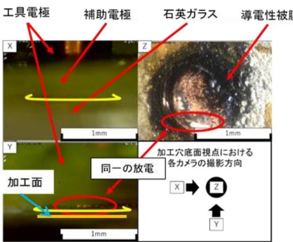
Fig. 8 Result of low energy discharge (1.7A)
