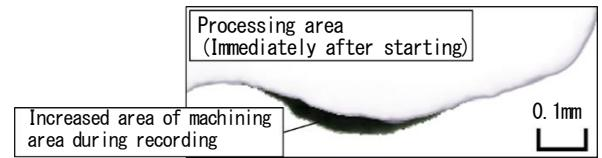
Fig. 4 Increased area of machining area during recording
