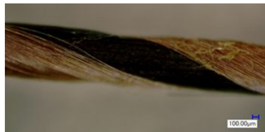
図6 An example of PBO filament covered carbon fiber bundle (SCCF)
