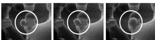
Fig. 2 - Droplet migration from the side to the top of the micropillar. Micropillar diameter and height is 50 micrometers.
