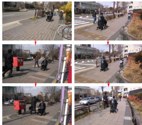
Fig. 7. On the left, the PMV first avoided a girl walking on the right side of the sidewalk after she avoided some bicycles. Then the PMV had to move back left to avoid incoming
