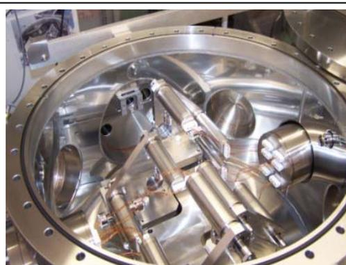
Fig.1 3D-4 mirror Optical Cavity in Vacuum
