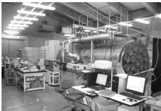
Fig. 2 NIES 6-m 3 photochemical smog chamber.
