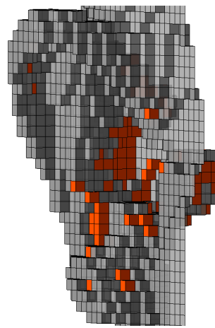
Fig. 2. Parts of the ear surface (colored) reduced in reflection coefficient to achieve the above results.
