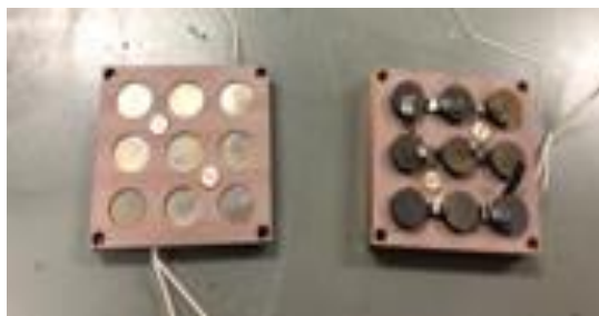
Fig.4 Photograph of the Thermoelectric module by using the \text{Mg}_2\text{Si} pelets synthesized under pressure.
