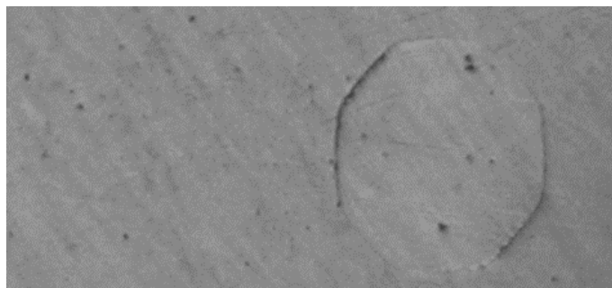
図3 Polarizing microscope image of nematic phase of 7CB in the homogenous alignment cell. Dotted circle shows the UV cured area by illumination for masked UV light using iris of fluorescent microscope unit.
