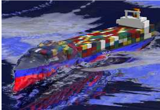
Fig.2 Example of computer graphics using computed results for wave-induced motions of S-175 container ship.
