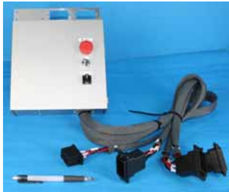
Fig. 10 Power supply switch circuit
