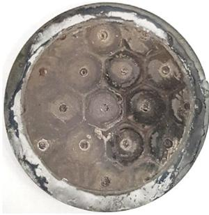
Fig. 2 Appearance photograph of  $MgB_2$  bulk produced by the MVT process. The central part is bulk  $MgB_2$  (diameter 20 mm, thickness 2 mm). The outer part is a reinforced steel ring. Hexagonal structures developed around circles corresponding to the Mg diffusion holes can be observed.
