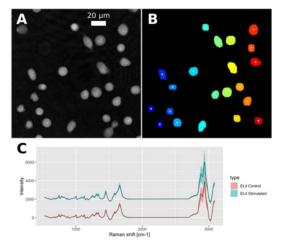
Figure 1: (A) Typical QPI image of EL4 T cells. (B) Automated segmentation of the objects in the field of view, where the center of each cells is used as an automatic target for the Raman laser excitation. (C) Typical average Raman spectrum of EL4 T cells with the standard deviation shown around the average (N=685).
