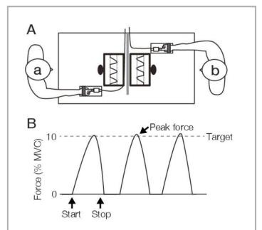
**Fig. 1.** Experimental setup **(A)** and definition and measurement of the dependent variable **(B)**. **A:** The individual condition used half of the setup; three joint conditions were executed by two individuals using the entire setup. **B:** The start and stop of force production were indicated by audible metronome. The interval between
