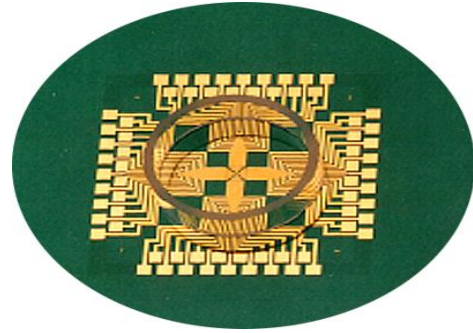
図1 集積化電極基板 (MicroElectrode Array: MEA)
