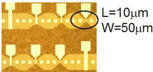
Fig. 1 Array of transistors with various channel sizes.
