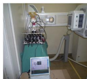
Fluoroscopic system used for VFSS simulation
