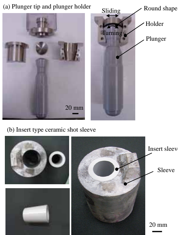
Fig. 12 Proposed hot-chamber injection system: (a) plunger tip and (b) insert type shot sleeve.
