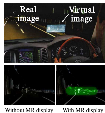
Fig. 1 MR environment for an advanced driver assistance system.
