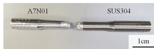
Fig. 5.2 A7N01/SUS304 joint after fracture.
