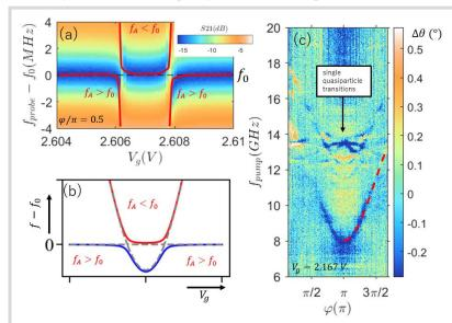
Fig. 4. (a) Single tone showing the response dispersive shift of the cavity resonance as successive ABSs are tuned to and through zero detuning with the cavity frequency. (b) Illustration of the cavity shift as the transition frequency  $f_A$ for excitation of the ABS is tuned rough the bare cavity frequency  $f_0$ . The sign of the
