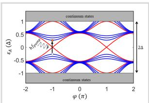
**Fig. 1.** (a) Illustration of ABSs energies  $\varepsilon_A$  for both trivial (blue) and topological (red) modes. The arrow indicates an example excitation of a trivial state with a microwave photon. The excitation frequency is  $f_A = 2\varepsilon_A/h$ .
