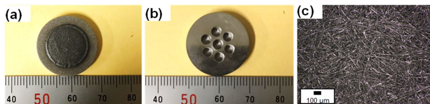
Fig.5 Developed MS-SOEC (a) anode side, (b) cathode side, (c) metal mesh layer.
