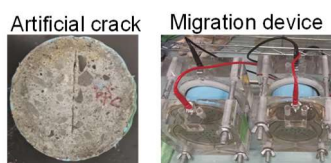
Fig. 3 Artificial crack and migration device
