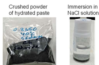
Fig. 6 Chloride binding test
