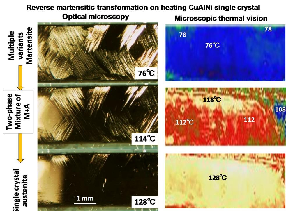
Fig.2 Martensitic transformation of the  $\beta_1'$  martensite forming the domains of the plate group variants.
