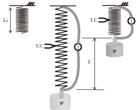
Measurement of helical spring actuation lifting weight up
