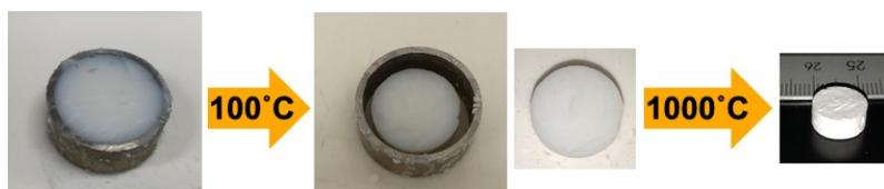
Fig. 2 Preparation process of macroporous calcium phosphate.
