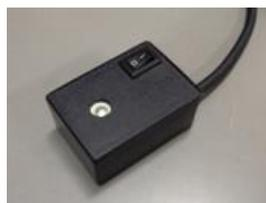
Fig. 2 GPS receiver for measurement of
