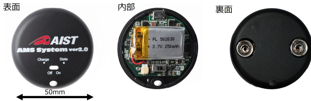
Figure 5: Compact terminal with integrated accelerometer and circuitry for generating muscle electrical stimulation signals
