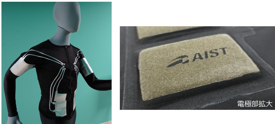
Fig. 3 Fabricated textile electrodes for EMS smart wear
