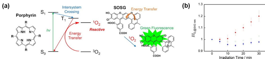
Fig. 2. (a) Schematic illustration of porphyrin-sensitized singlet oxygen generation and its reaction with SOSG. (b) fluorescence intensity ratio I/I_0 at 540 nm ( \lambda_{\text{em}} = 540 \text{ nm} , \lambda_{\text{ex}} = 509 \text{ nm} ) as a function of photoirradiation time at 420 nm observed for SOSG alone (green, control) and SOSG with porphyrin nanowires fabricated by the irradiation of 6 with 490 MeV ^{192}\text{Os}^{30+} particles at the fluence of 1.0 \times 10^{10} \text{ cm}^{-2} (blue) and 1.0 \times 10^{11} \text{ cm}^{-2} (red).
