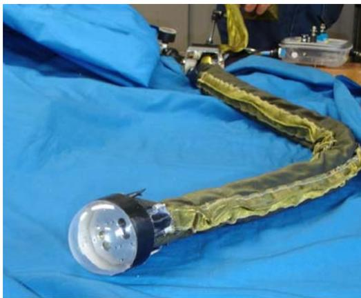
Fig.4 Overall view of Grow-hose-I with a head unit on its tip
