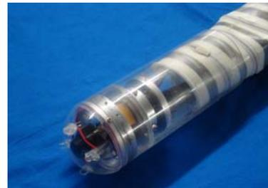
Fig.6 Developed head unit equipped with a camera, LEDs, and the driving mechanism.
