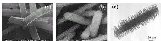
Fig. 1 SEM & TEM images of (a) hexagonal and (b, c) screw-like ZnO nano rods prepared by heating  $\text{Zn}^{2+}$ -HMT aqueous solution at  $95^\circ\text{C}$  for 3 and 76 h, respectively.
