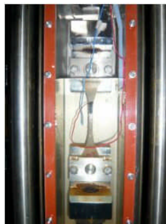
Fig. 3 Experimental setup for constant tensile load tests in hydrothermal environment.
