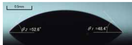
Fig. 10 Contact angle at the critical condition when droplet starts to slide ( \alpha MSD, A=3.8\mu\text{m} , output of Laser=20mW)
