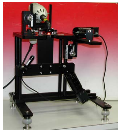
Fig.1 Laser speckle contrast measurement system
