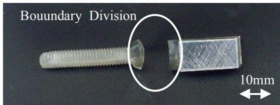
Fig. 3 Tensile fracture specimen in pull-out test.
