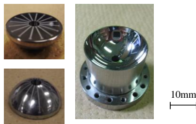
Fig. 2 Photographs of spherical bearing parts for actuator
