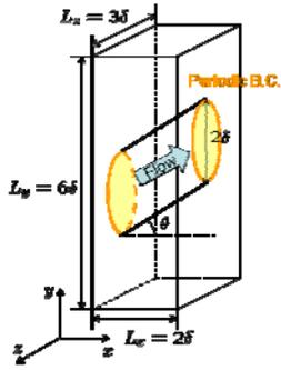
Fig. 1. Schematic diagram of the arrangement of cylinder in the computational domain
