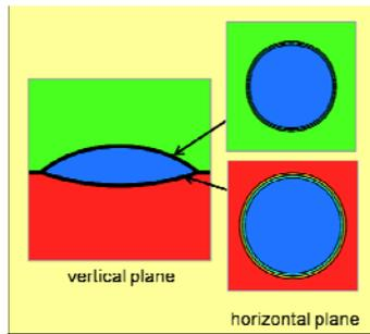
Fig.8 Steady state shape of the droplet (blue) in two different fluid interfaces (red and green). Contour lines on the cross sections indicate diffuse interface region.
