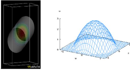
(a) Velocity vector (b) Profile of the axial direction velocity
