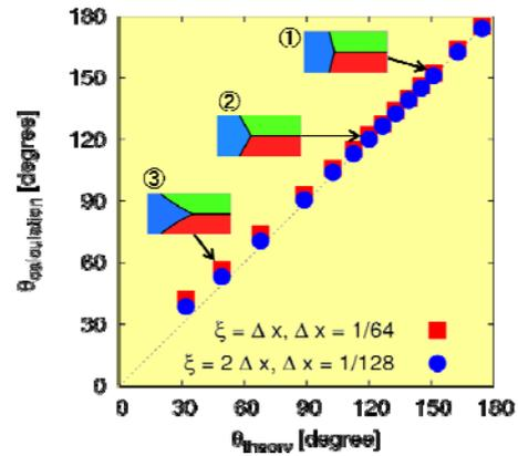
Fig.6 The represented contact angle of blue fluid at triple junction as function of the theoretical contact angle. Symbols are compared for the resolution of the diffuse interface.
