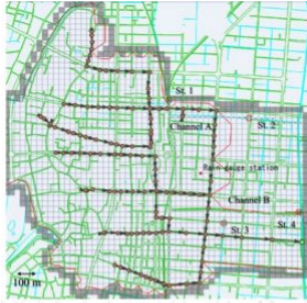
Fig. 4 Structure of the adopted NILIM model 11) with one dimensional sewers and two-dimensional overland flows.
