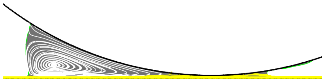
Fig. 6 Enlarged view of oil film profile with streamline in vane with zero gravity
