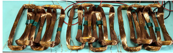
(b) Coil of the rotor
