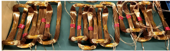
(b) Coil of the stator
