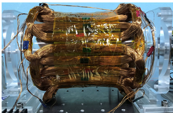
(c) Stator of experimental prototype
