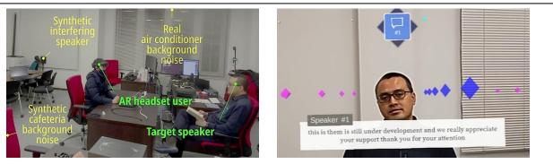
Figure 3: We developed a prototype system with augmented reality smart glasses (Microsoft HoloLens 2). The left figure illustrates one of the evaluation setups and the right figure depicts the smart glasses user point of view showing some virtual markers and transcription of the enhanced speech.
